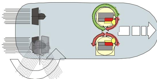
Turn the starboard or port propulsor through 180°; the starboard propulsor counter-clockwise or the port propulsor clockwise, i.e. turn the control levers from ahead to astern, via zero position.
